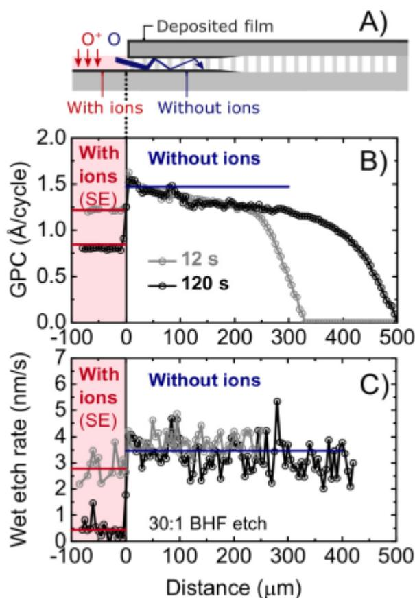
**Fig.1.** LHAR channel structures (a) with which the GPC (b) and wet etch rate (c) of PE-ALD SiO<sub>2</sub> films grown with and without the ion contribution. [4]
